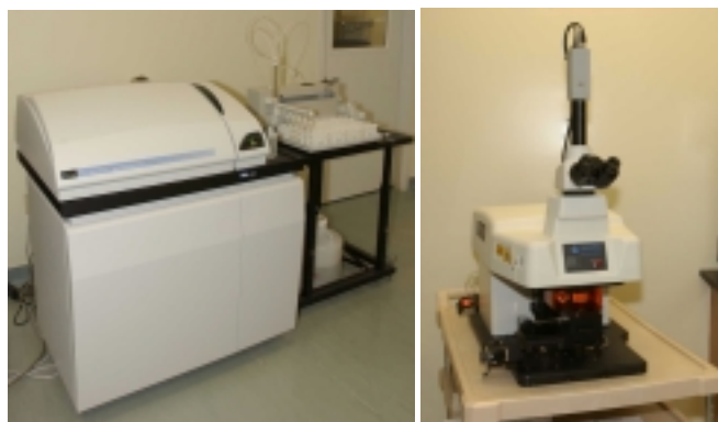
Fig. 1. Perkin Elmer ELAN DRC II ICP-MS (a) and New Wave Research Nd:YAG LA ( \lambda = 213 \text{ nm} ) unit (b)
